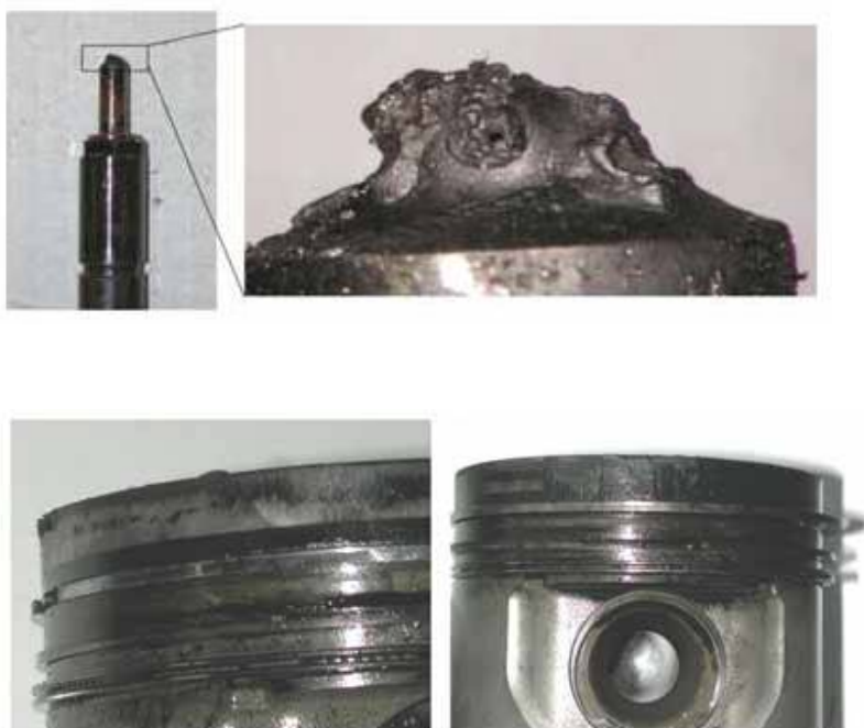
Picture 5.1: Carbon Deposits at Injector Nozzle and at Piston Rings
